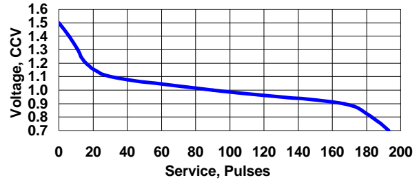
PULSE TEST 1.8 ohms - 15sec/min 24 hours/day
